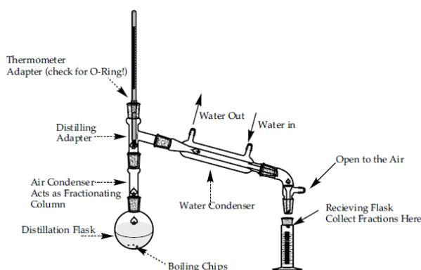
1. Assemble distillation apparatus as shown in diagram.
