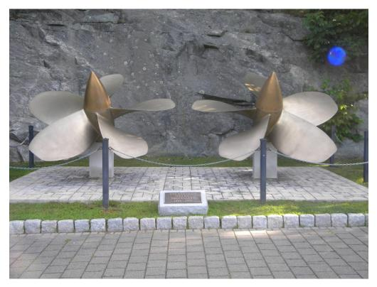
The twin propellers from USS *Nautilus* (SSN 571) at the Submarine Force Museum, Groton, CT. USS *Nautilus* was the first nuclear-powered ship, using the energy from the fission or "splitting" of the Uranium 235 atom to generate heat from a nuclear reactor core, which in turn heated water to make steam to spin turbines to rotate the propellers.
