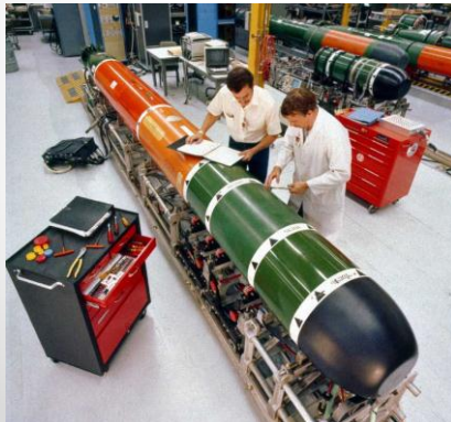
- Keyport Technicians working on a Mark 48 in early 1982 - Mark 48 ADCAP torpedo aboard USS Asheville (SSN-758)
